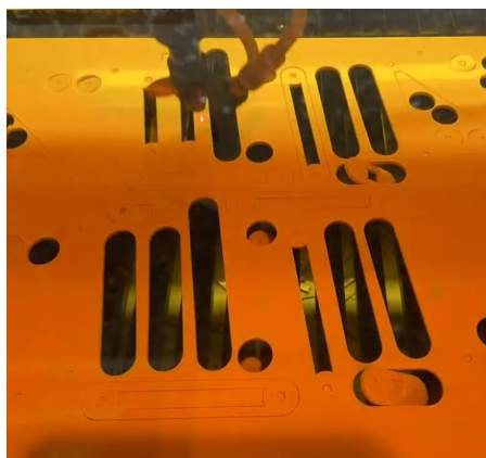
Appendix E.1: Laser cutting the two sets of flat ground legs
