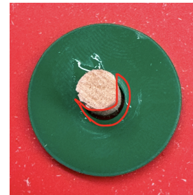
Figure 29: Dowel - dowel cover spacing issue
