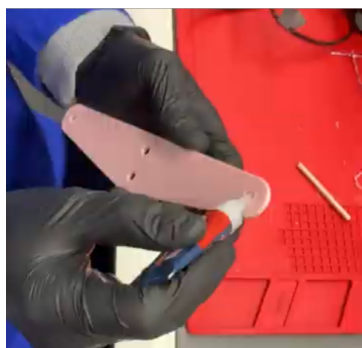
Appendix E.3: Glueing the longest dowels at point D on our original diagram onto the base which holds the legs together
